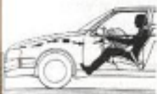
The sensor has registered the decrease in speed and sends a signal to a gas generator, via the control module, which inflates the airbag.
