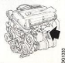
Engine number stamped on the engine block
