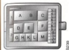
Arrangement of fuses on panel at back of glove compartment
