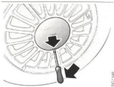
Removing the hub cap
