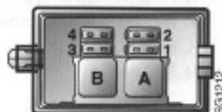
Arrangement of fuses on panel at back of glove compartment
