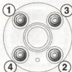
Tightening sequence for wheel studs
